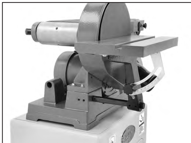
Figure 34. Installing work table onto table support rod.
